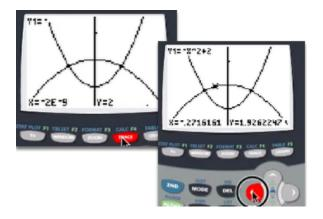
2. Use the Up or Down arrow keys to switch functions. Then use the Right and Left arrow keys to trace.
